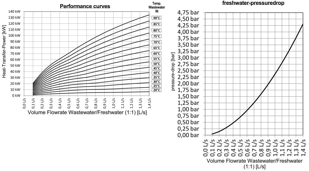
(250527) Datasheet - FERCHER Wastewater-Heatexchanger Type FB-1 - Characteristic curves
