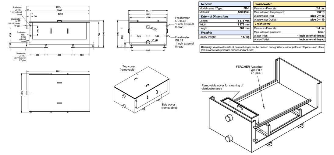
(250527) Datasheet - FERCHER Wastewater-Heatexchanger Type FB-1 - Dimensions and data, all measures in millimeters
