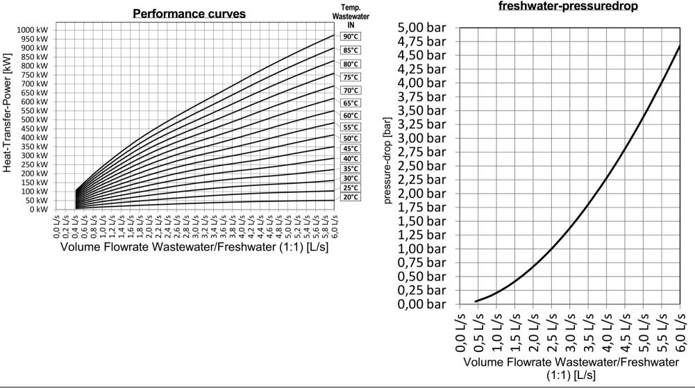
(250527) Datasheet - FERCHER Wastewater-Heatexchanger Type FB-12/W-2-2 - Characteristic curves
