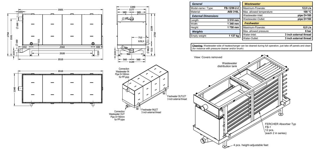
(250527) Datasheet - FERCHER Wastewater-Heatexchanger Type FB-12/W-2-2 - Dimensions and data, all measures in millimeters
