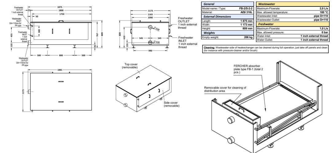
(250527) Datasheet - FERCHER Wastewater-Heatexchanger Type FB-2/S-2-2 - Dimensions and data, all measures in millimeters
