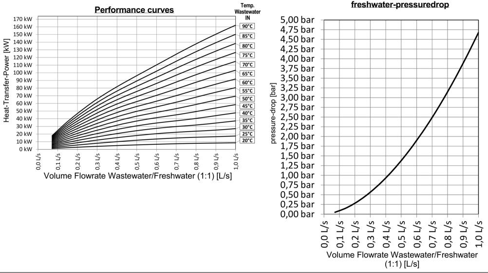
(250527) Datasheet - FERCHER Wastewater-Heatexchanger Type FB-2/S-2-2 - Characteristic curves
