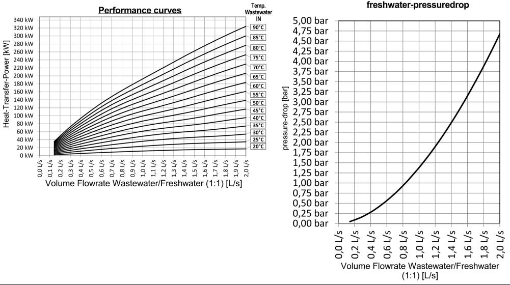
(250527) Datasheet - FERCHER Wastewater-Heatexchanger Type FB-4/S-2-2 - Characteristic curves
