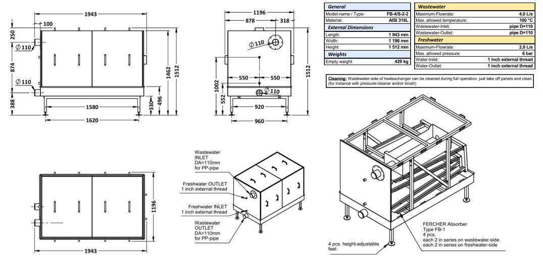
(250527) Datasheet - FERCHER Wastewater-Heatexchanger Type FB-4/S-2-2 - Dimensions and data, all measures in millimeters
