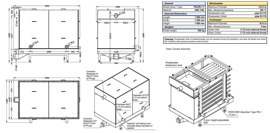
(250527) Datasheet - FERCHER Wastewater-Heatexchanger Type FB-6/S-1-1 - Dimensions and data, all measures in millimeters
