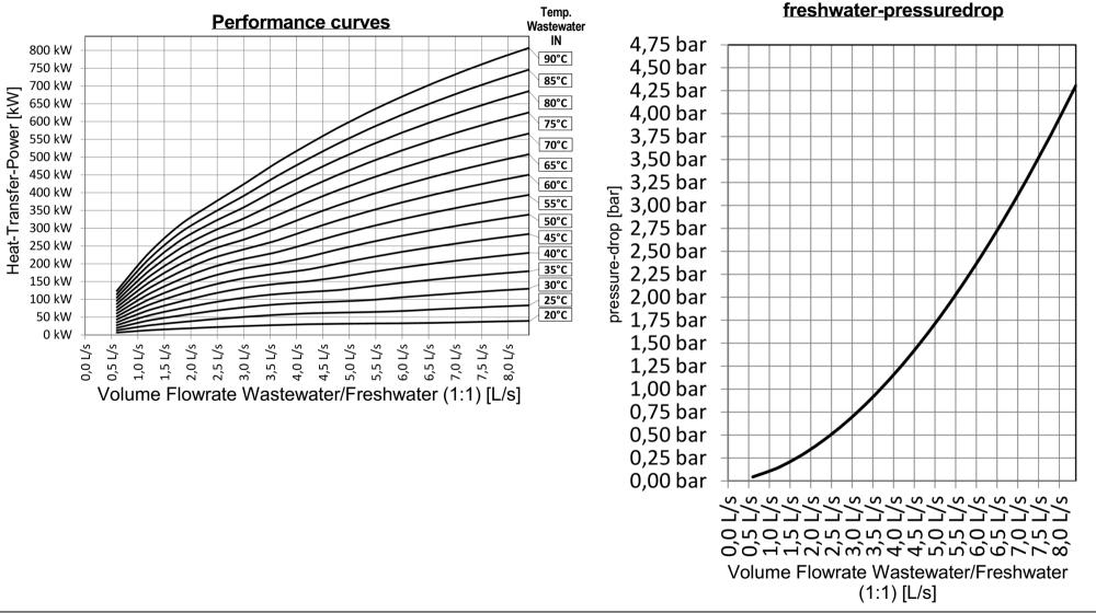
(250527) Datasheet - FERCHER Wastewater-Heatexchanger Type FB-6/S-1-1 - Characteristic curves
