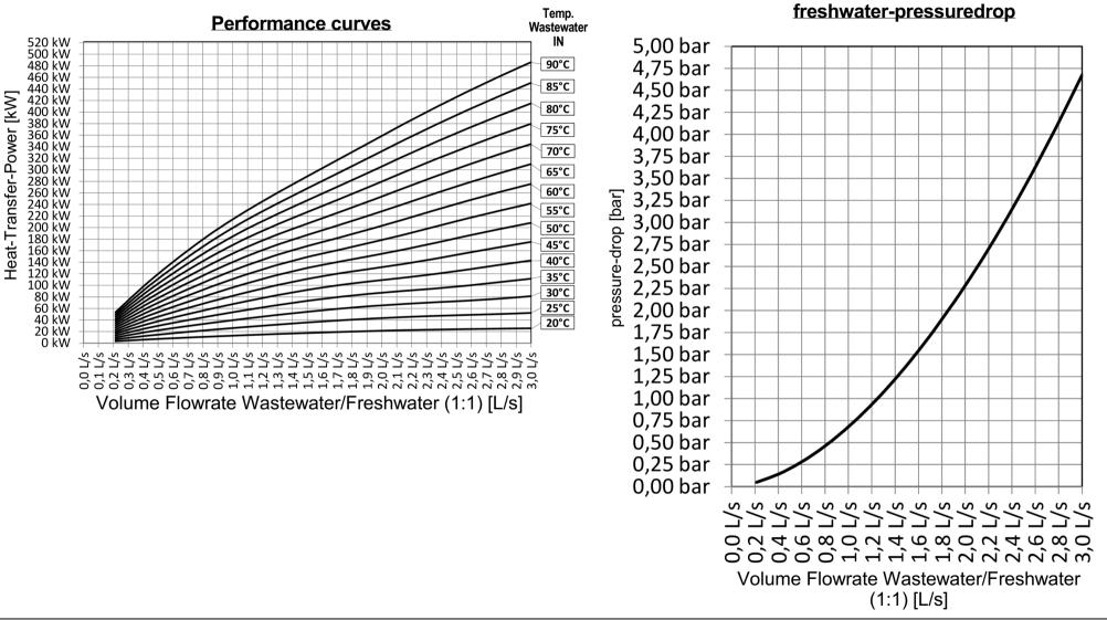
(250527) Datasheet - FERCHER Wastewater-Heatexchanger Type FB-6/W-2-2 - Characteristic curves
