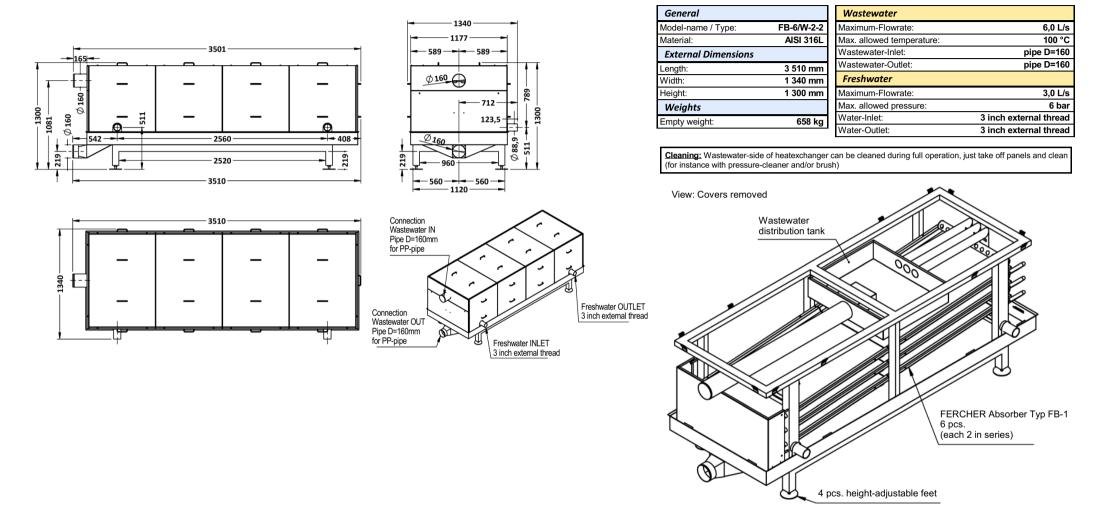
(250527) Datasheet - FERCHER Wastewater-Heatexchanger Type FB-6/W-2-2 - Dimensions and data, all measures in millimeters
