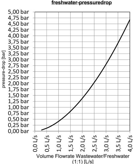
(250527) Datasheet - FERCHER Wastewater-Heatexchanger Type FB-8/W-2-2 - Characteristic curves
