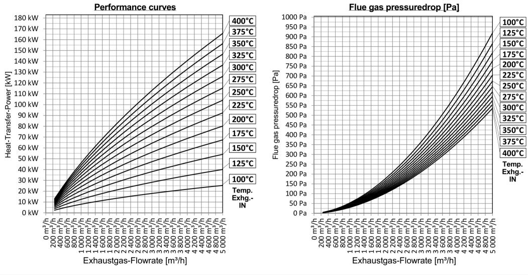
(250430) Datasheet - FERCHER flue gas heatexchanger type FW-400 - Characteristic curves
