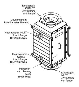
(250430) Datasheet - FERCHER flue gas heatexchanger type FW-400 - Dimensions and data, all measures in millimeters
